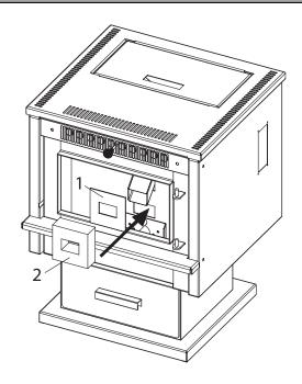
3. Install the auger chute gasket as shown. Place the thin gasket (1) first and the thicker gasket (2) second.
