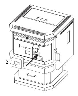
3. Install the auger chute gasket as shown. Place the thin gasket (1) first and the thicker gasket (2) second.
