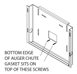
4. When placing the back heat shield back in place, ensure that the bottom edge of the thick auger chute gasket sits on top of these 2 screws.
